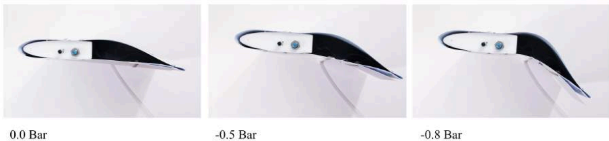
Figure 30: Airfoil prototype bending at various negative pressures.
