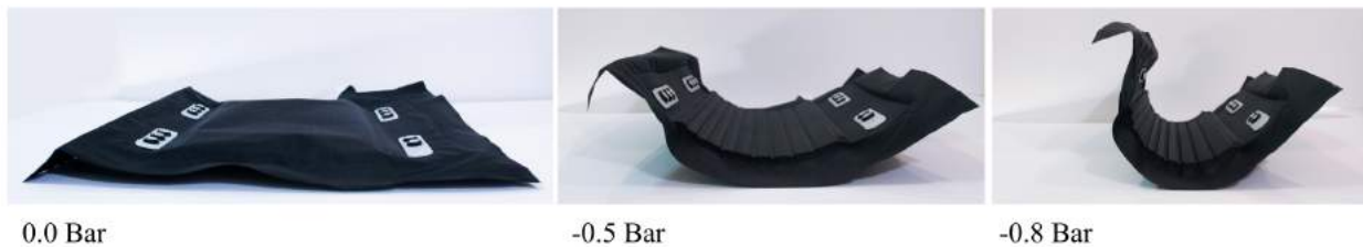
Figure 26: First prototype of actuating airfoil surface interior. Though this prototype was sufficiently rigid, the second iteration included taller ridges to improve the stability of the airfoil shape in high windspeeds.
