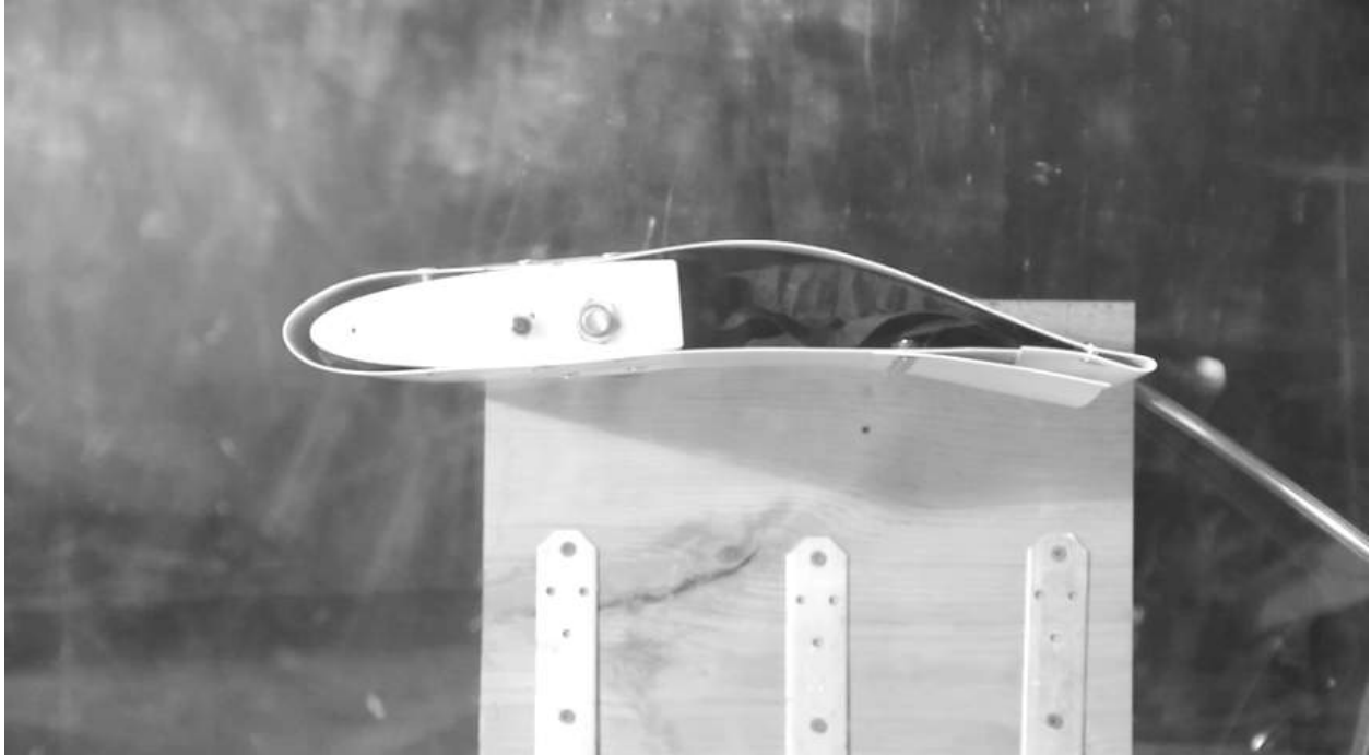
Figure 28: Airfoil prototype in the wind tunnel
