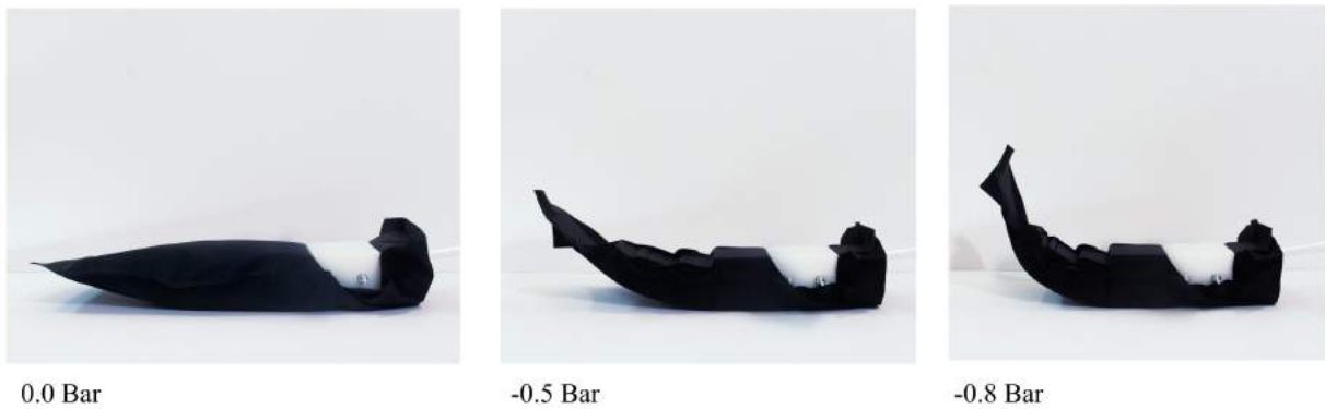
Figure 27: Prototype of the interior of the morphing airfoil.
